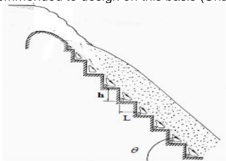
Figure 1. Flow on the stepped spillway
